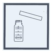
Pour the contents of the tube into the square mixing bottle.
