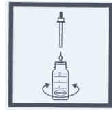
While swirling the mixing bottle, add Hardness 3 Titrant solution drop by drop. When the sample changes from red to blue, record the number of drops added.
